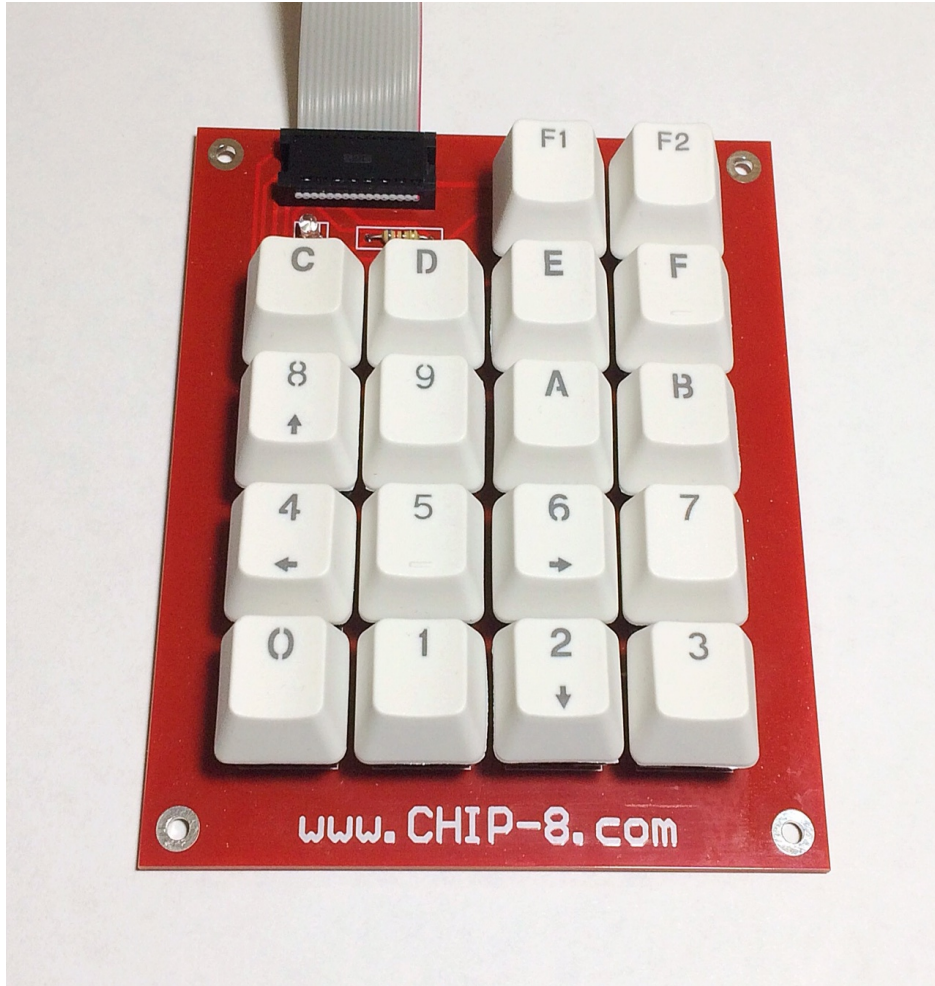
Figure 2: CHIP-8 Hexadecimal Keypad
