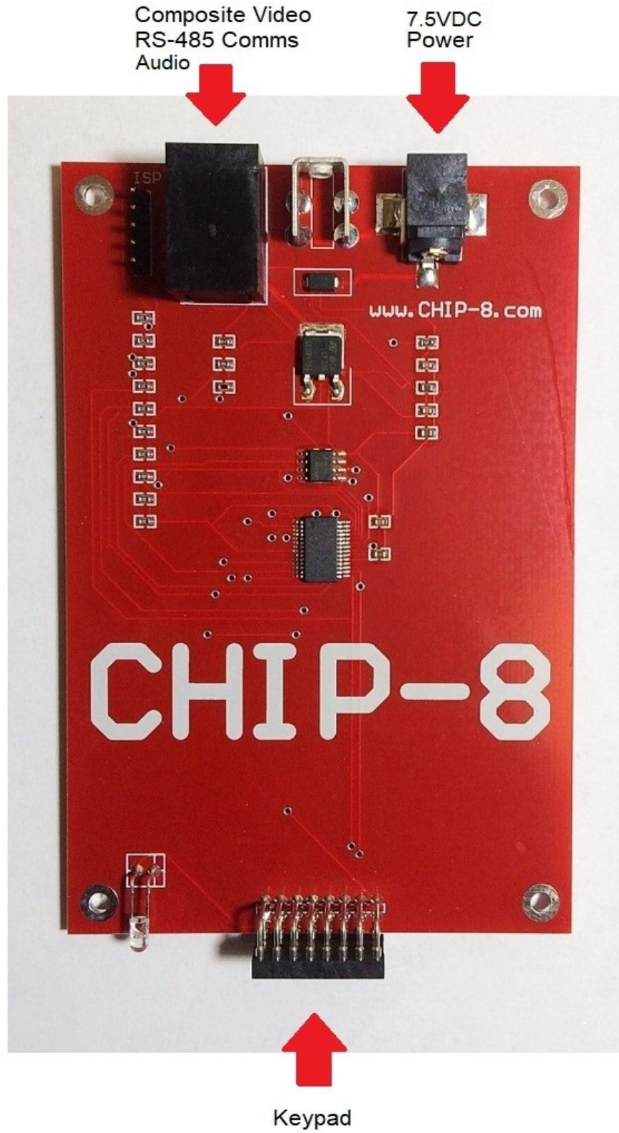
Figure 1: CHIP-8 Interface Connectors
